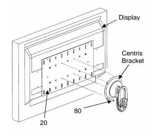
Figure 11. Attach Display to Mount
